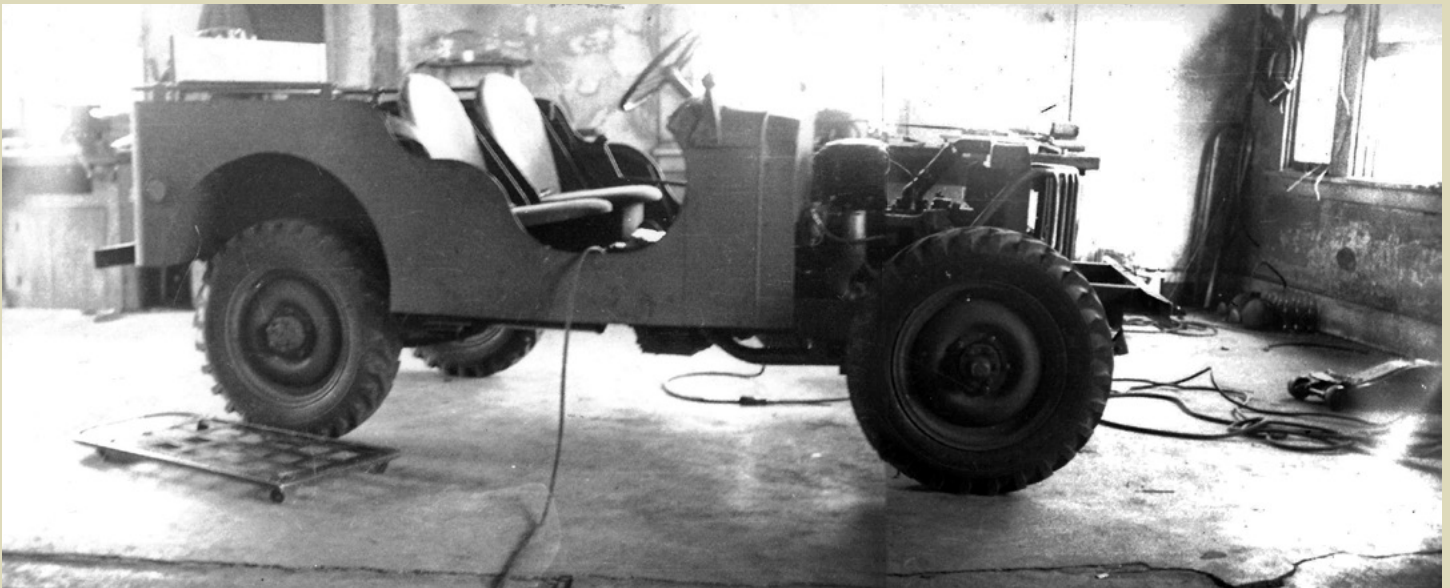
The body tub is mounted on the chassis. Note the extension cords, likely used for portable tools and work lights, as well as the mechanic's creeper in the photo.
