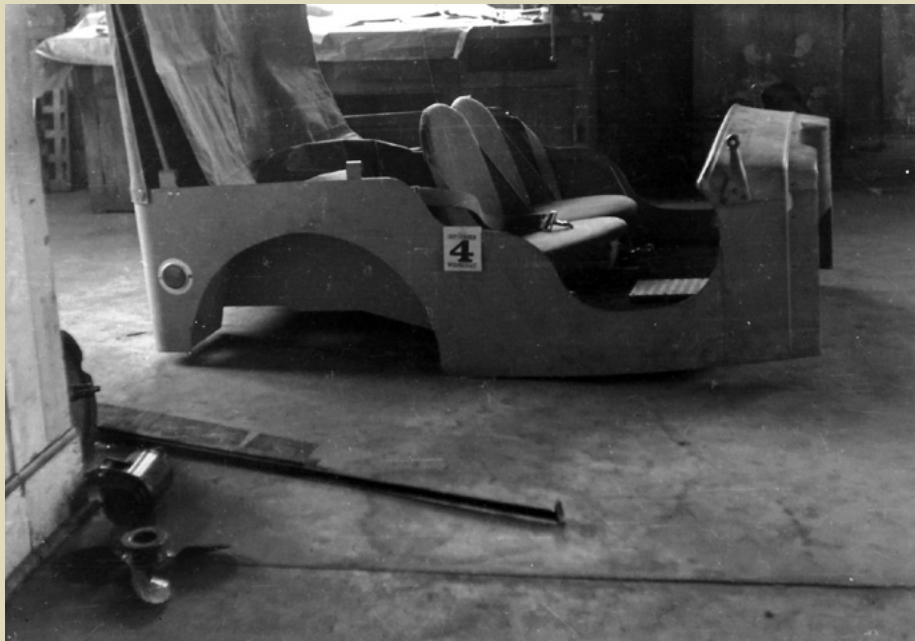
September 4, 1940. The body tub assembly, complete with canvas-upholstered seats, awaits its fitting to the chassis. This tub was hand built by Ralph Turner and Chet Hempfing.
